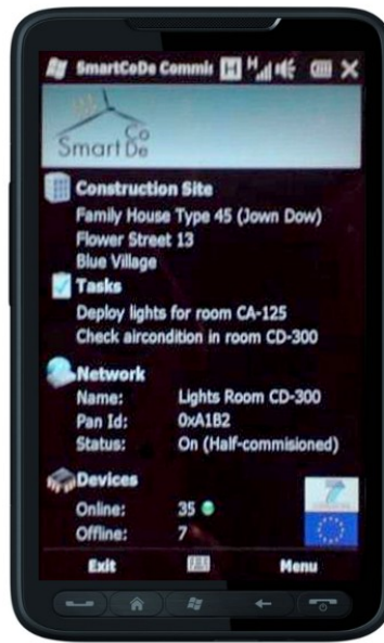
Figure 1.3.10: The SmartCoDe commissioning tool
