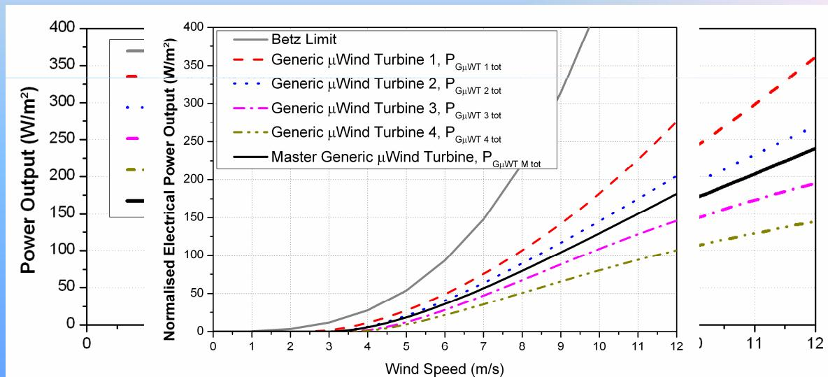
$$P_{\text{G}\mu\text{WT } M \text{ tot}} = (1 - e^{-0.75(v-3)})(-7.87v + 2.92v^2 - 0.084v^3), \text{ for } v \geq 3 \text{ m/s}$$
