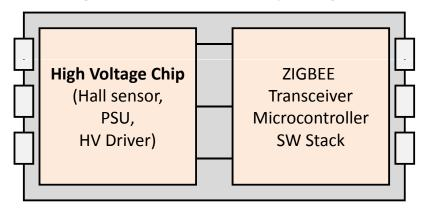
"Dies" (=Silicon chips) are in one package, connected by bonding wires
